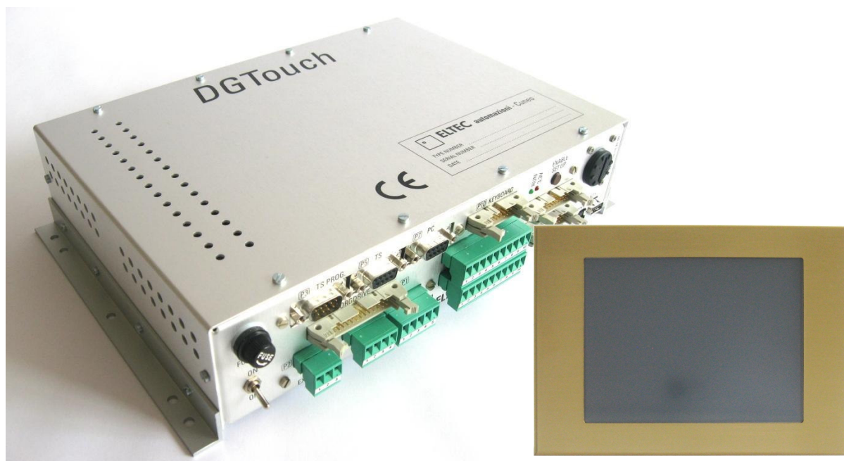
Base unit PROGRAMMER for the installation in console (Code PROGINT ) with display TFT touch screen 5,7' plate (Code PD5.7).
